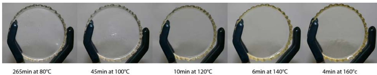
Figure 14. Photos and cure times of DER 354 and Lindride 52D with Hycat™ AO-4 at 2.0% loading at varying cure temperatures
