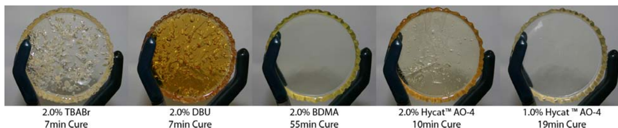
Figure 5. Photos and cure times of Lindoxy 190 and Lindride 52D with different catalysts at 2.0% loading at 120°C. Photo on the far right is the same resin mixture with AO-4 at 1.0% loading for visual and cure time comparison.
